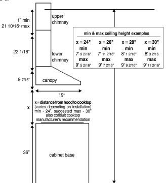
For ducted installations the chimneys are adjustable and designed to meet varying ceiling heights between 7' 9 2/16" and 9' 11 2/16" depending on the distance between the bottom of the hood and the cooktop (distance x in the ducted diagram).
